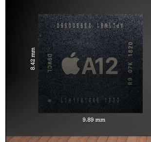
9<sup>th</sup> Generation Apple-designed processor Debuted on iPhone XS First commercial 7nm mobile processor 6.9 Billion Transistors 2.49 GHz 64-Bit ARM Architecture
